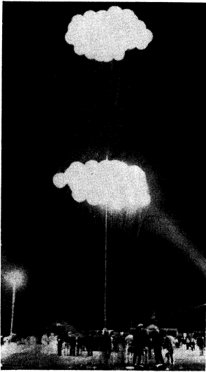
Multiple-balloon aerostat used by Jean Piccard in 1937 at Rochester, Minn.
