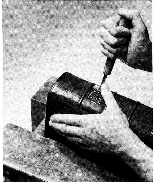
9. Tooling the title on the spine with handle letters through gold leaf
