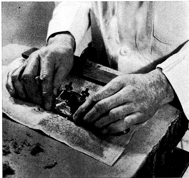
7. Paring the inner surface of the covering leather with a spokeshave
